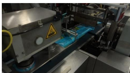
Figure 27 - Packing Machine (lengthwise sealing)
