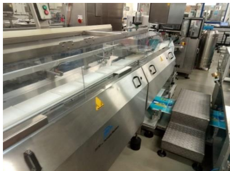
Figure 26 - Packing Machine (loading conveyor)
