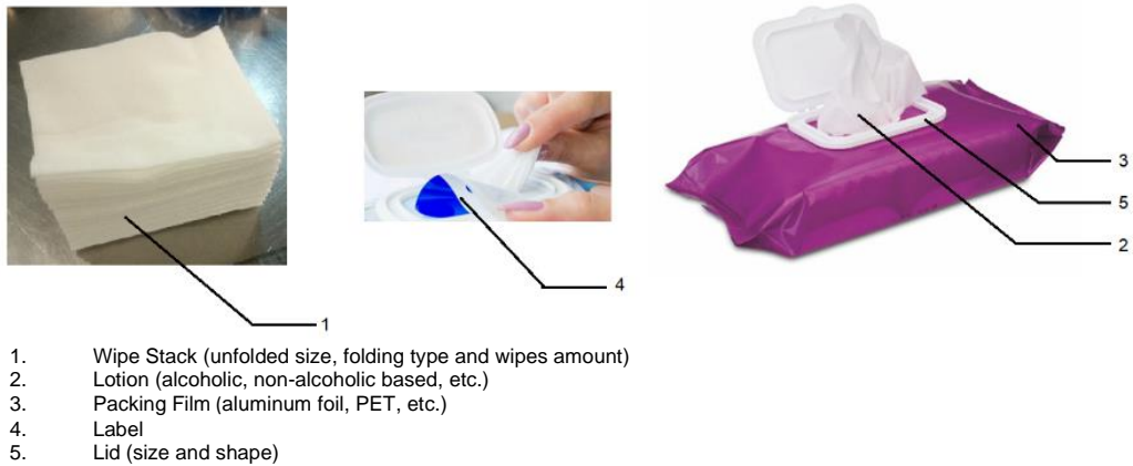
Figure 18 - Basic components of a package
