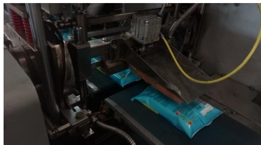
Figure 28 - Packing Machine (latitudinal sealing)
