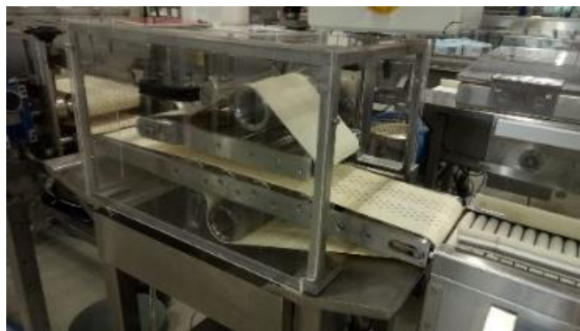
Figure 24 - Pressing unit (stage)
