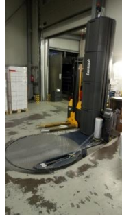
Figure 34 - Stretch wrap machine (stage)
